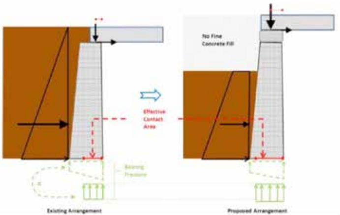
Figure 1 Proposed deck heavier than existing.
