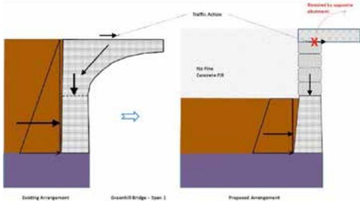
Figure 3 Greenhill bridge span 1 reconstruction.
