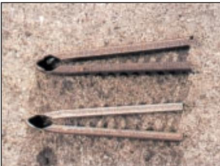
Only AL1 spikes can be fitted in conjunction with spikelocks. If AL23s are used the spikelock will be driven right through the base of the sleeper.
