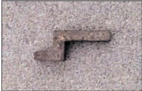
Where a gap is wide the appropriate expansion bit is dropped in, the rails can be closed up by the adjuster onto the bit, the rail fastened down and the bit knocked out. If a number of gaps have bits placed in them then one position of the adjuster can be sufficient to correct all of them at the same time.
