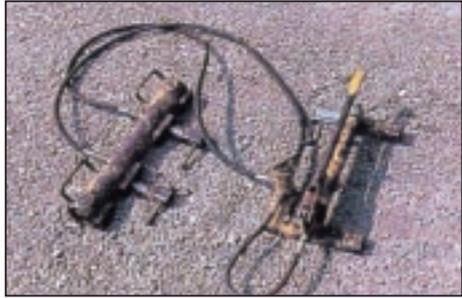
Expansion bits corresponding to the 3, 6 and 10mm gaps can easily be made from pieces of steel of appropriate thickness and are helpful when used with the hydraulic adjuster.
