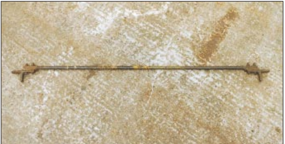
Fig.4. Gauge-setting bar NOT a track gauge
