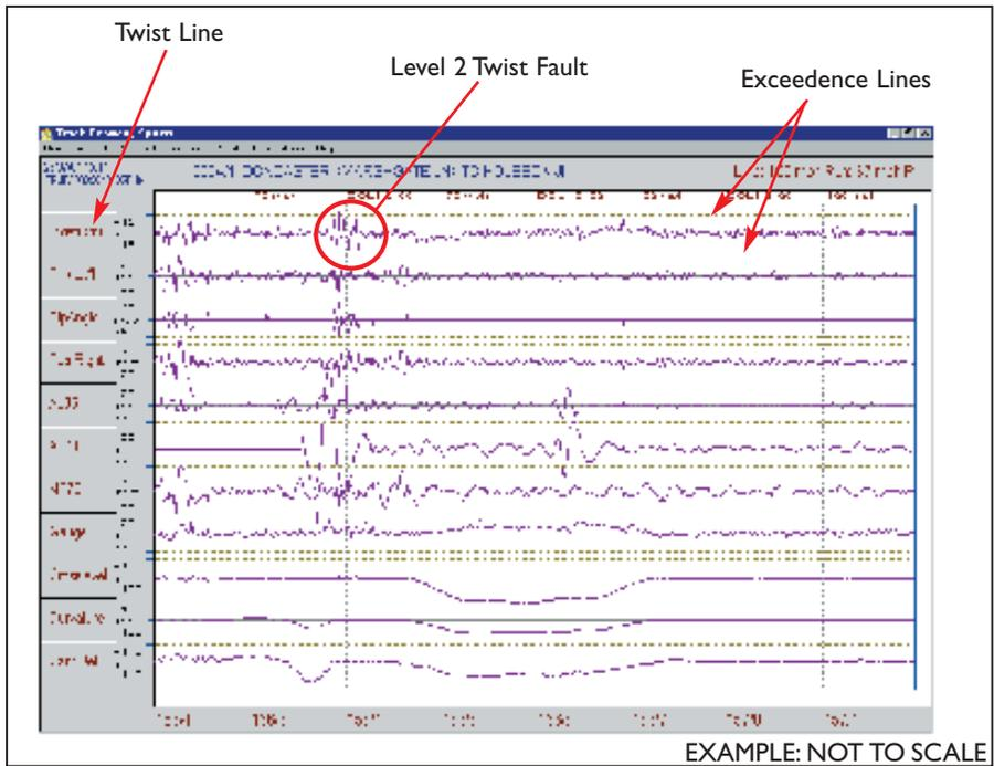
The computers on-board the TRV monitor and process all the data collected by the measuring systems. In addition to twist these systems record data for top, alignment, cant deficiency, dynamic gauge, cross-level and curvature and others listed in the left hand column of the chart.
