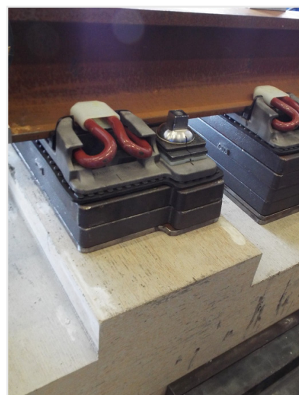
Image 3: Baseplates under test at +70 mm and +140 mm adjustment
