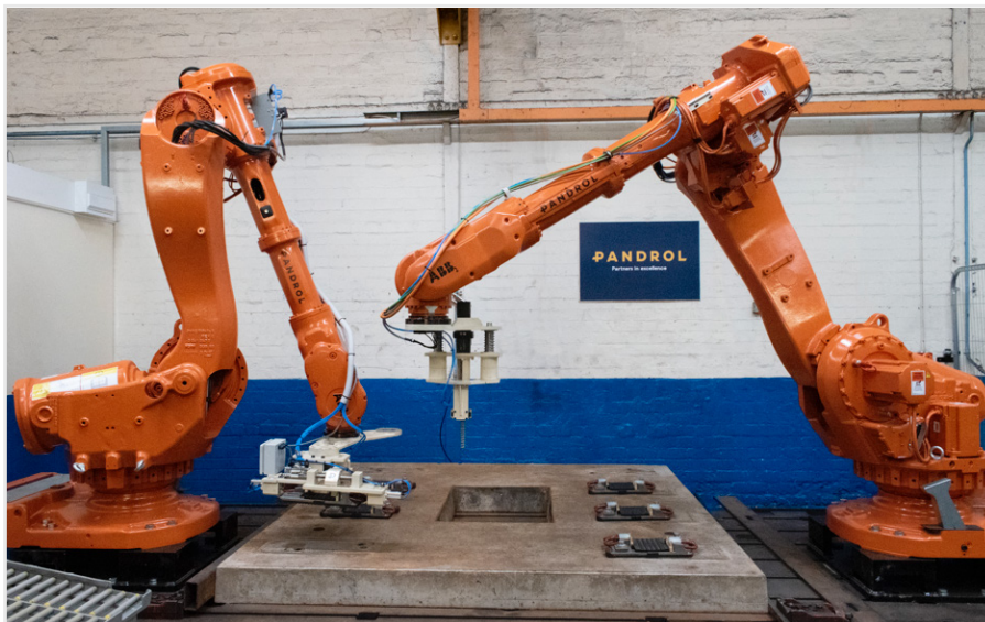
Image 1: Robots Installing baseplates
