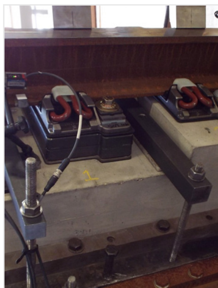
Image 2: Baseplates under test at +0 mm and +70 mm adjustment
